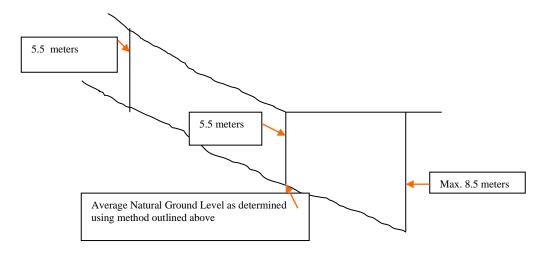
At any point on the erf the maximum eaves height is 1,5m below the maximum roof height at that point.
